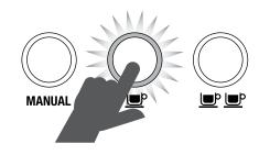
The machine will stop after 1 CUP volume has been extracted and will return to STANDBY mode.
